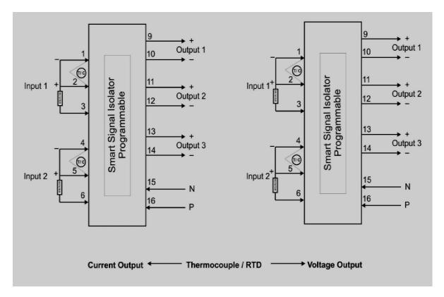
Connection Diagram: Thermocouple & RTD
