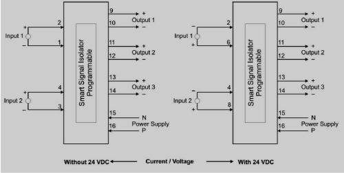
**Connection Diagram: Current & Voltage**
